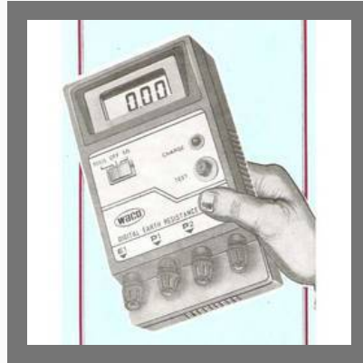
Digital Earth Resistance Tester
